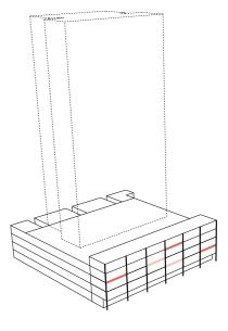
Figure 71: Vertical proportions reinforced by structural grid Irregular balcony rhythm set within the regular column grid
