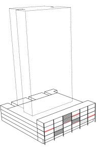
Figure 72: Infill screens, louvres and solid panels alternate within the structural grid
