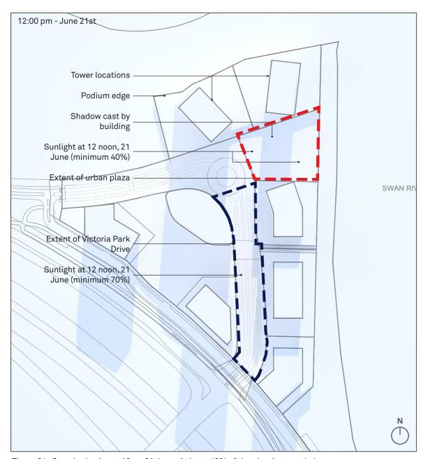
Figure 64: Overshadowing at 12pm 21 June. At least 40% of the plaza's ground plane and at least 70% of Victoria Park Drive's ground plane shall be in sun at 12pm on 21 June.
