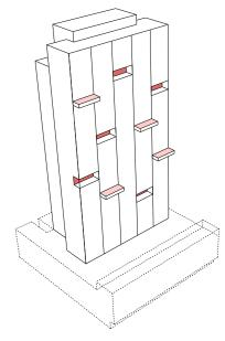
Figure 75: Vary balcony treatment with recessed and protruding elements to give facade depth
