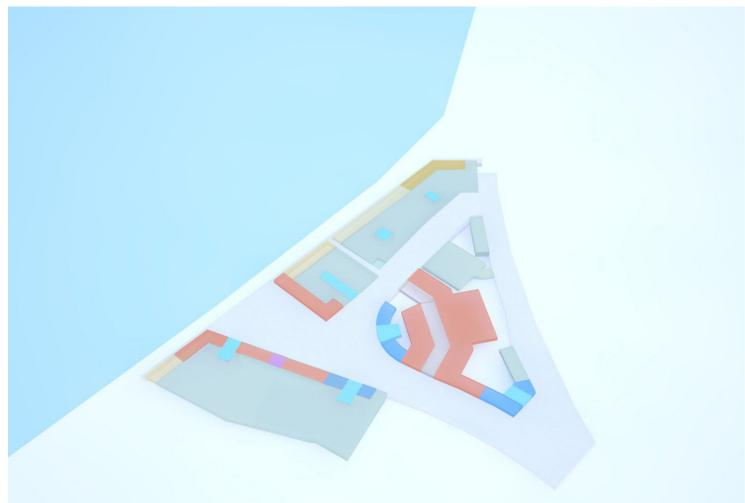
Figure 15: Ground floor land uses at or near plaza / Seabiscuit Drive level. Exact levels will vary at time of development. A minimum finished floor level of 3.7 metres AHD shall apply for occupiable floor space throughout Precinct D, whilst development will also need to be within 1.2 metres of the adjacent finished footpath level. Basements for parking, building services and store areas shall be permitted below 3.7 metres AHD.
