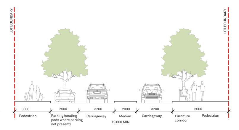
Figure 85: Section describing the characteristics of Victoria Park Drive. Note: drawing is notional to help describe general requirements and intended function.
