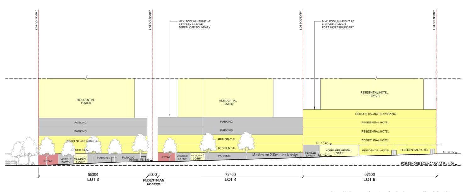
Figure 80: Demonstration of stepping development up Victoria Park Drive on lots 3,4 and 5. Note: The land uses described in these drawings are indicative and for explanatory purposes only. For specific criteria, refer to the Specific 45 Building Requirements.
