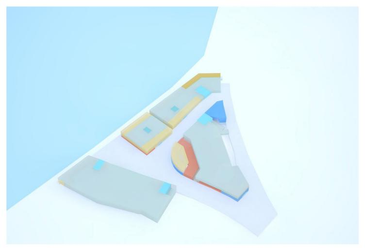
Figure 18: Ground, first, second and third floor land uses above. This describes the general principle of how car parking is to be sleeved by occupied floor space, and where car parking is intended to extend to the building edge at upper levels (which has less impact on the character of the street).
