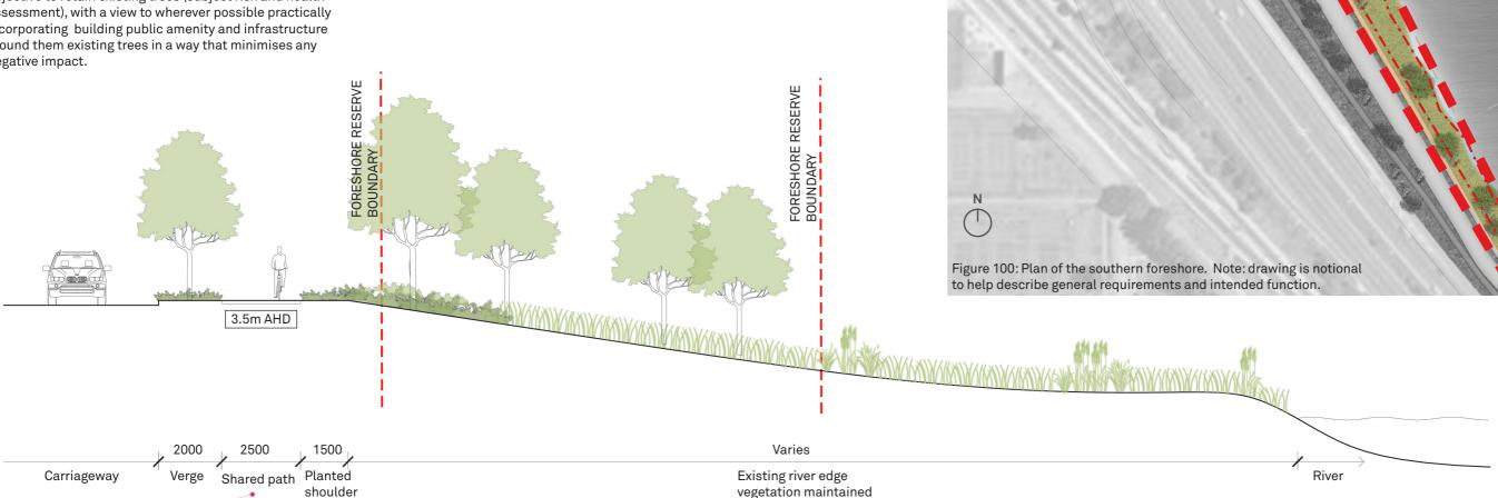
Figure 101: Section drawing of the southern foreshore in the area indicated. Note: drawing is notional to help describe general requirements and intended function.
