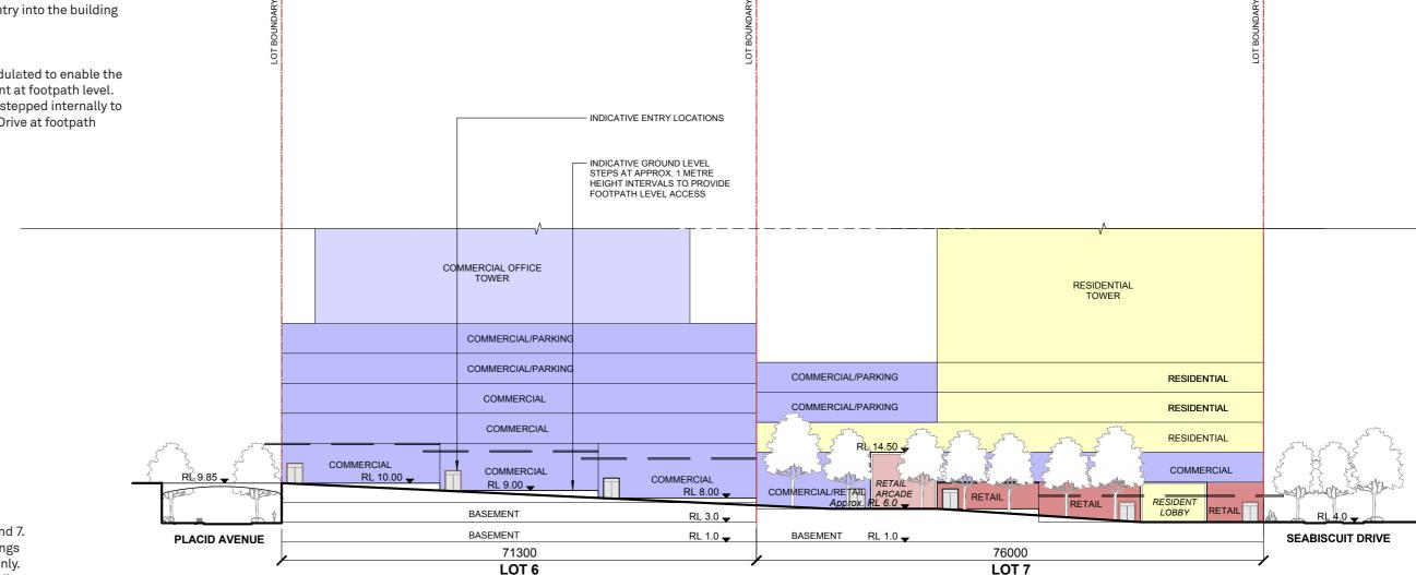
Figure 79: Demonstration of stepping development up Victoria Park Drive on lot 6 and 7. Note: The land uses described in these drawings are indicative and for explanatory purposes only. For specific criteria, refer to the Specific Building Requirements.
