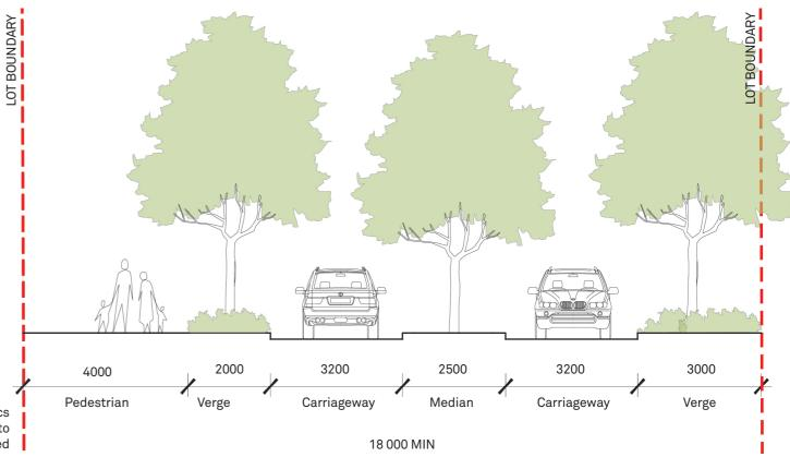
Figure 92: Section describing the characteristics of Seabiscuit Drive. Note: drawing is notional to help describe general requirements and intended function.
